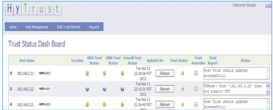
Figure 8. Trust Status Dashboard Indicating Two Trusted and One Untrusted Host
