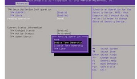
Step 11: Advanced > Trusted Computing > Pending Operation > Enable Take
